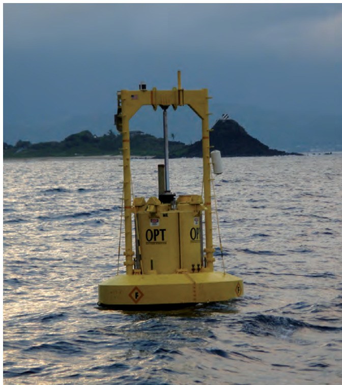
Buoy type WEC off the coast of Hawaii Image courtesy of Ocean Power Technologies, Inc.
